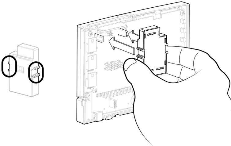
3. Carefully press the front housing with installed WiFi module back on to the backplate.
