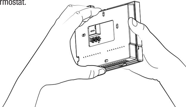
2. Install the Wi-Fi module as shown onto the printed circuit board.
